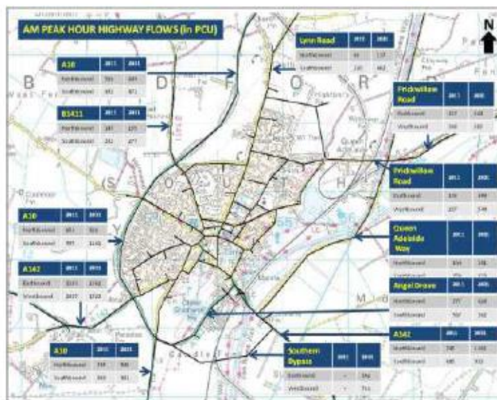
©Crown Copyright 2012- Cambridgeshire County Council OS Licence Number 100023205 Figure 4: Changes in highway link flows in the morning peak between 2011 and 2031. Source: East Cambridgeshire Local Plan Transport Test (October 2012).
