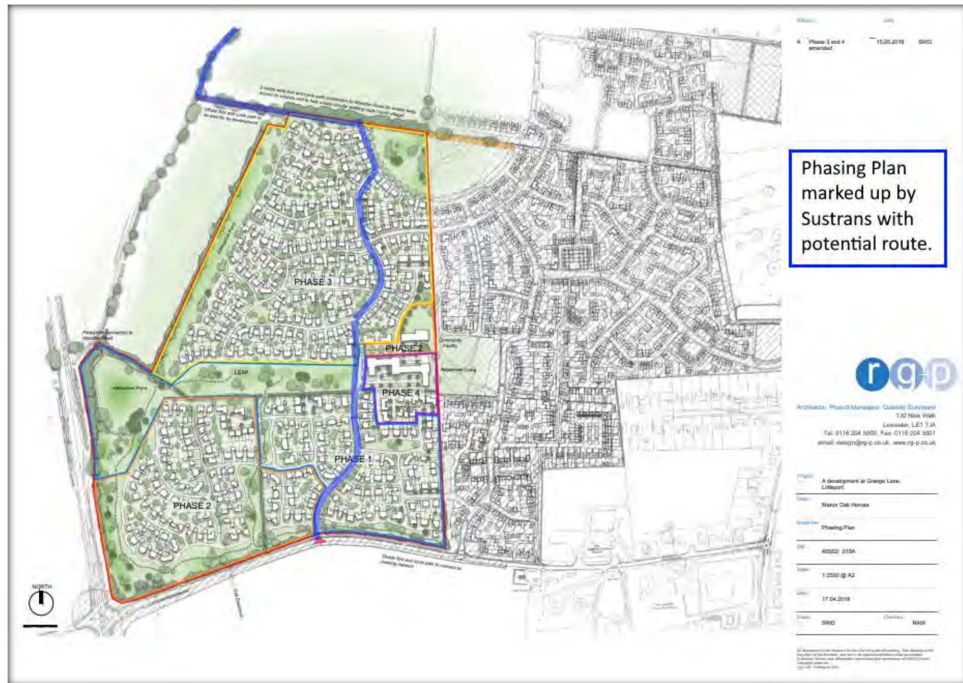
Figure 7.1.15.1 Phasing Plan for developments north of Grange Lane, with blue route alignment marked on by Sustrans. Note that the route is for a link with Woodfen Road not the route to the centre of Littleport, which is shown in Figure 7.1.16.1.
