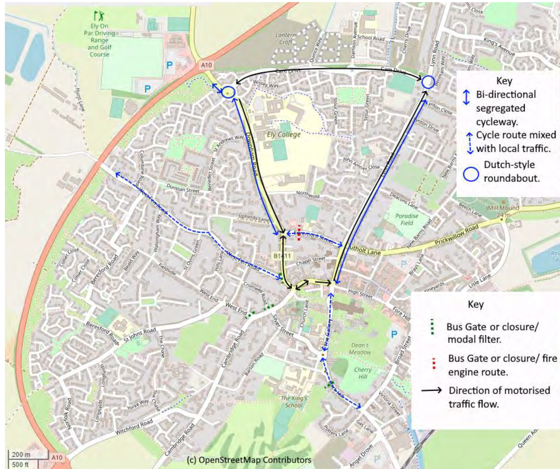
Plan showing possible traffic flows and cycleway provision assuming one-way systems and bus gates are introduced as above. Note that no detailed design or consultation has been done, but an indicative design for the Dutch style roundabout has been prepared to show that this should be feasible. (See following page).
