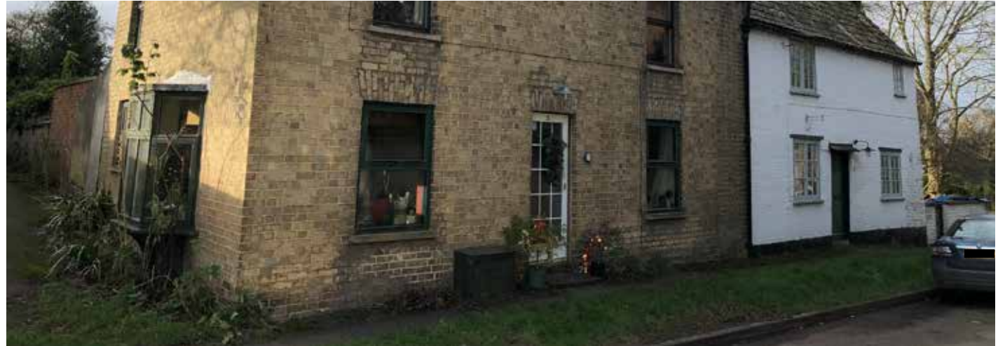
Figure 49: Windows on side elevations (left) can increase natural surveillance and sunlight inside houses.
